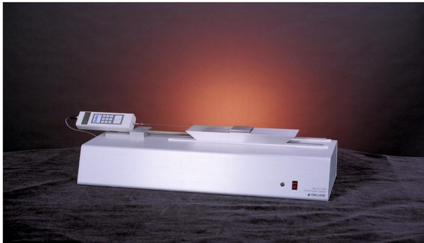
*The Model FX-7100 Film Coefficient of Friction Tester.*
