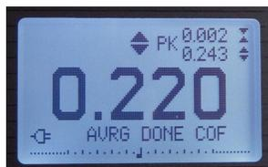
*Digital Console Display Showing Measured Kinetic and Static COF Values*
